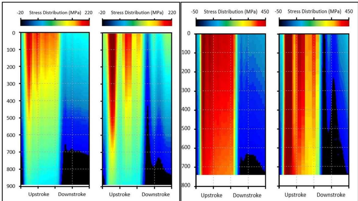
Figure 5. Stress distribution for wire rope in the slanted well (left box) and vertical well (right box), low speed/production (on the left) and high speed/production (on the right) inside each box
