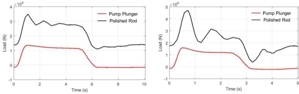
Figure 3. Wire Rope in a slanted well, low speed/production (left), high speed/production (right)
