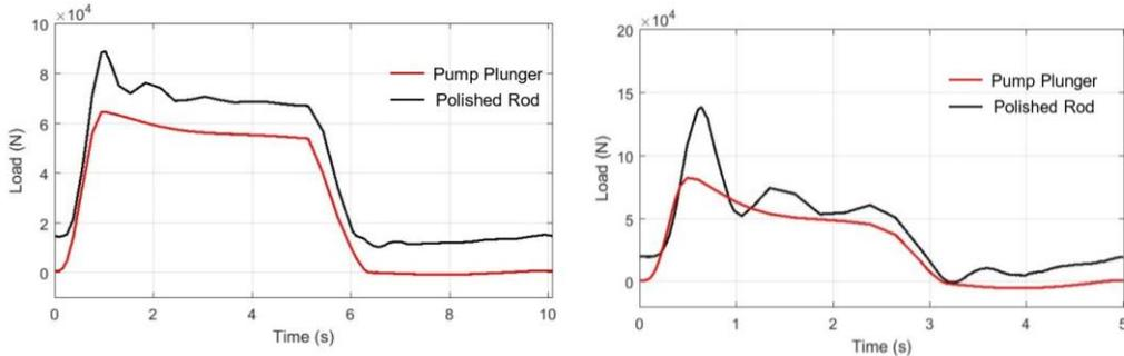
Figure 4. Wire Rope in a vertical well, low speed/production (left), high speed/production (right)
