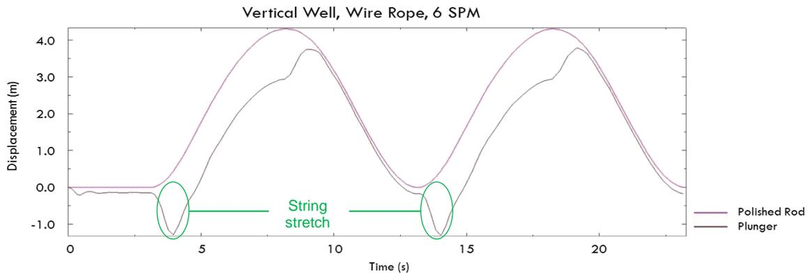
Figure 2. String stretch in the CSR, in vertical well and with low SPM
