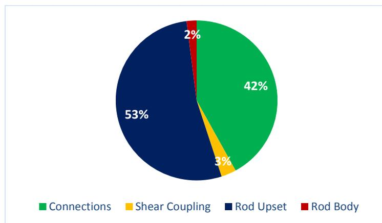
Figure 1. Failure Distribution by Location [3]
